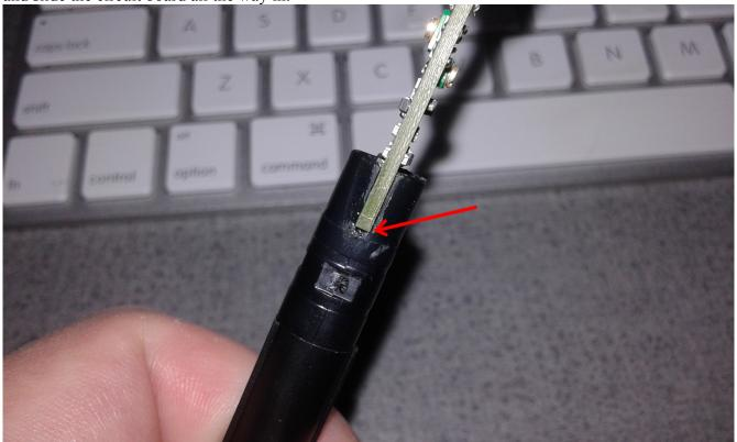
Don't use too much glue, and wipe off any excess before it dries, as it will get in the way when you reassemble the pen. IMPORTANT: Wait until the glue is completely dry before you reassemble the pen, otherwise closing it up will be permanent. It's a very tight fit.
