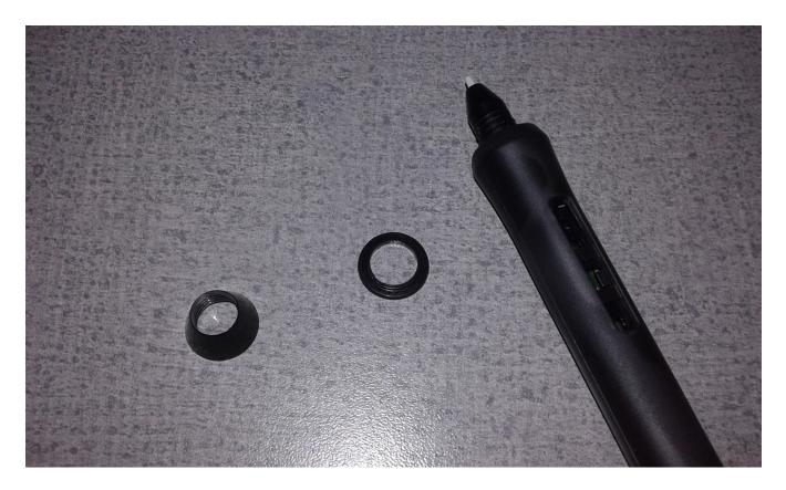
Step 3: Remove the rubber grip by sliding it down off the pen.
