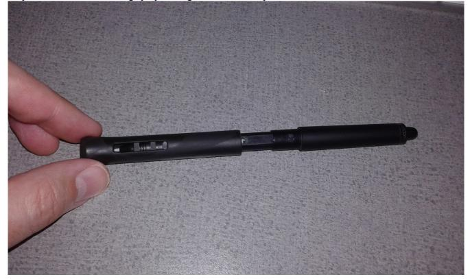
Step 4: NOTE: There is a tiny TINY SUPER TINY MICROSCOPIC little spring in the eraser end between the cap and the sensor, be very careful not to lose this when you separate the pen body...
